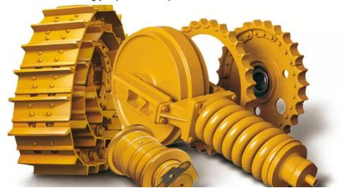
Undercarriage track roller is made of shell, bronze bushing, collar, seal, lock pin, plug, shaft. It is made by forging, machining, heat treatment, assembly, painting etc. The quality and working
